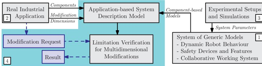
**Fig. 1.** The internal structure of the introduced safety concept for HRC systems. It contains of the four phases defined by (1) Modelling, (2) Analysis, (3) Identification, and (4) Operation.
