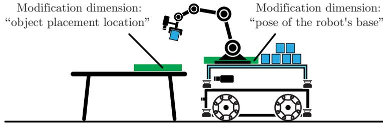
Fig. 3. Simplified representation of two exemplary modification dimensions
