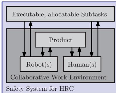
**Fig. 2.** Simplified work system model for HRC safety evaluation
